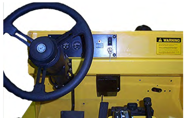
Dash and Instrument Panel shown above is equipped with optional Tilt/Telescoping Steering Column.
