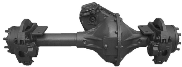
Heavy duty drive axle with high capacity disk brakes.
